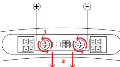
RIMUOVERE LED ESISTENTE / REMOVE LED
