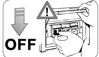
**BEWARE:** Connecting the fitting when power is on could irremediably damage the LEDs.
